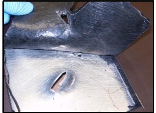
Figure 7: Exit Wound Wall Displaced [3]
