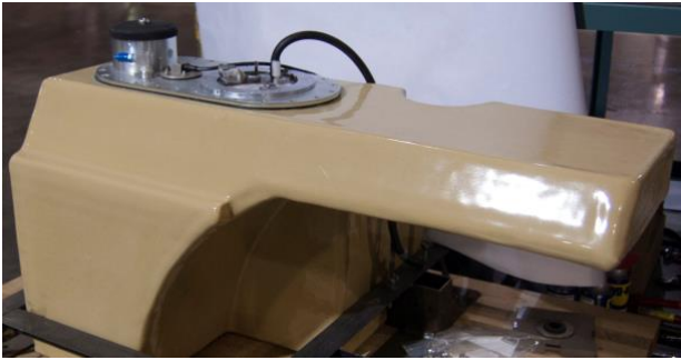
Figure 3: Space Optimized Plastic Fuel Tank [3]
