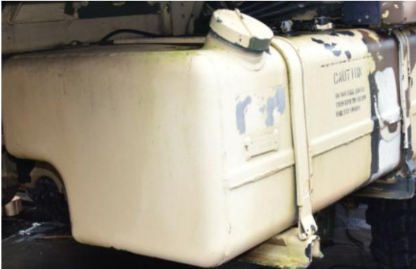
Figure 2: Aluminum Fuel Tank
